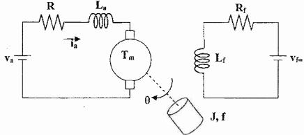
Choose the armature current  $i_d$ , the angular displacement of shaft  $\theta$ , and the speed  $\frac{d\theta}{dt}$  as state variables and  $\theta$  as output variables. (16)
