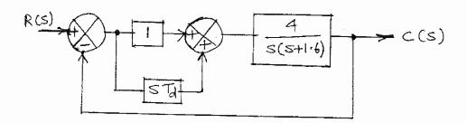
Determine the value of  $T_d$  so that system will be critically damped. Calculate its settling time. (8)
